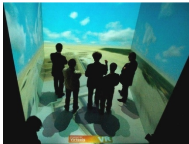
Figure 6. CAVE virtual reality display.
